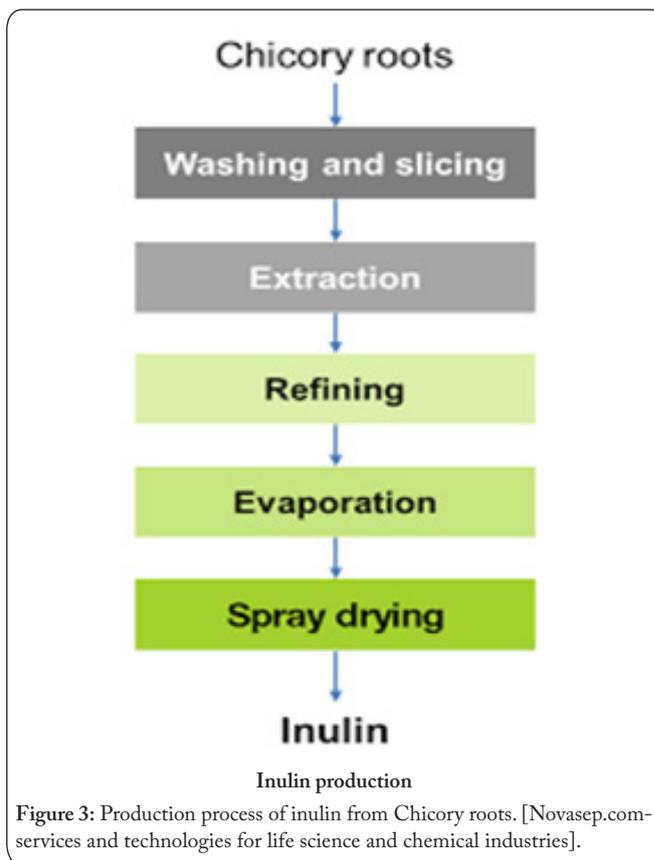
**Figure 3:** Production process of inulin from Chicory roots. [Novasep.com-services and technologies for life science and chemical industries].
