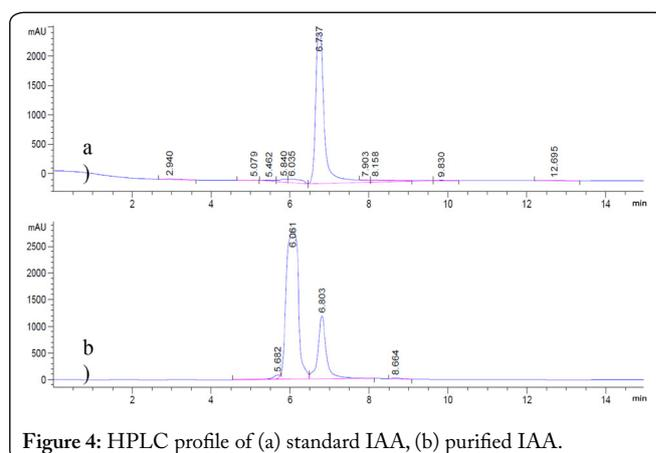
Figure 4: HPLC profile of (a) standard IAA, (b) purified IAA.
