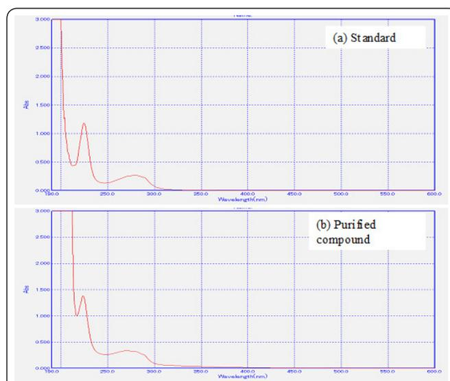
Figure 3: UV-Visible spectrum of IAA: (a) standard IAA (0.01 mg/ml); (b) purified compound from *P. chrysosporium* (100 times diluted fraction).
