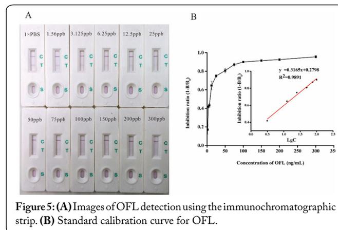
**Figure 5:** (A) Images of OFL detection using the immunochromatographic strip. (B) Standard calibration curve for OFL.
