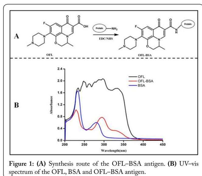
Figure 1: (A) Synthesis route of the OFL-BSA antigen. (B) UV-vis spectrum of the OFL, BSA and OFL-BSA antigen.
