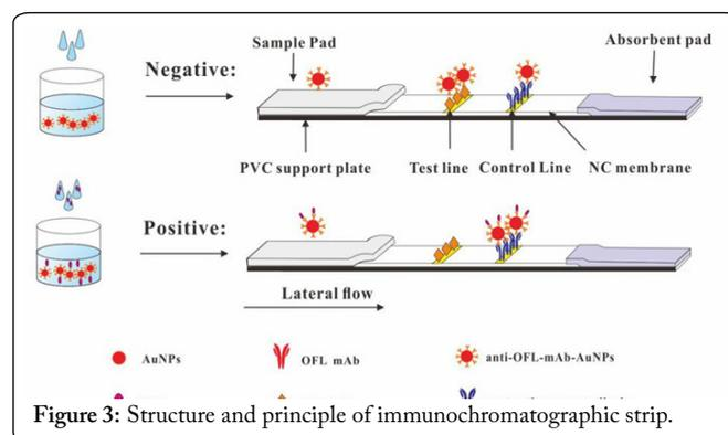
Figure 3: Structure and principle of immunochromatographic strip.
