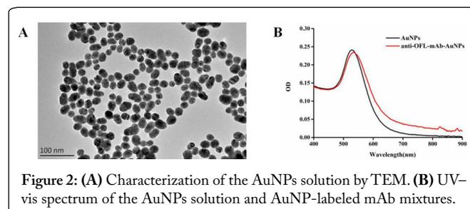
Figure 2: (A) Characterization of the AuNPs solution by TEM. (B) UV-vis spectrum of the AuNPs solution and AuNP-labeled mAb mixtures.
