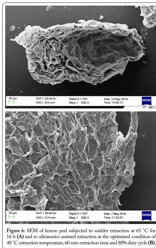
Figure 6: SEM of lemon peel subjected to soxhlet extraction at 65 °C for 16 h (A) and to ultrasonics assisted extraction at the optimized condition of 48 °C extraction temperature, 60 min extraction time and 80% duty cycle (B).
