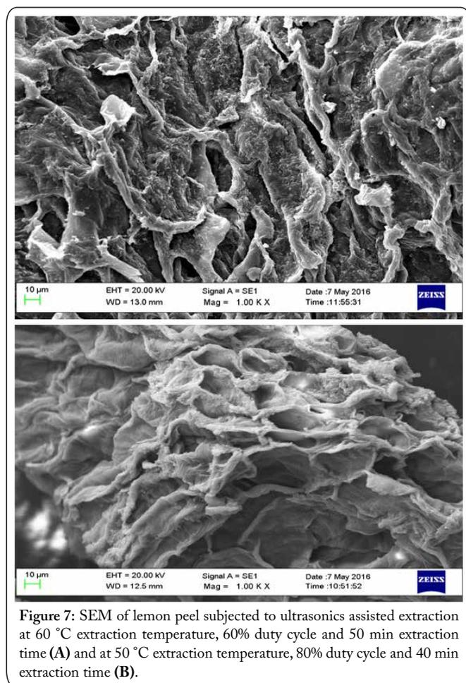
**Figure 7:** SEM of lemon peel subjected to ultrasonics assisted extraction at 60 °C extraction temperature, 60% duty cycle and 50 min extraction time (A) and at 50 °C extraction temperature, 80% duty cycle and 40 min extraction time (B).
